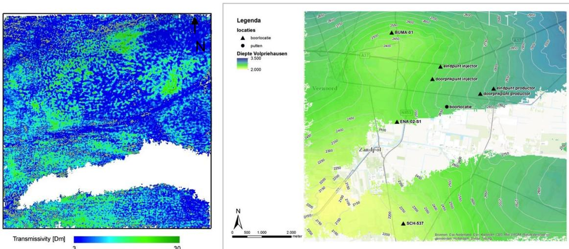
**Figure 2: The transmissivity (Dm) of the proposed geothermal Lower Volpriehausen geothermal reservoir was calculated with log and 3D seismic data analysis (left). From the surface location horizontal wells at aquifer depth are drilled in NE direction into top Volpriehausen reservoir(right) (Heijnen et al., 2010).**
