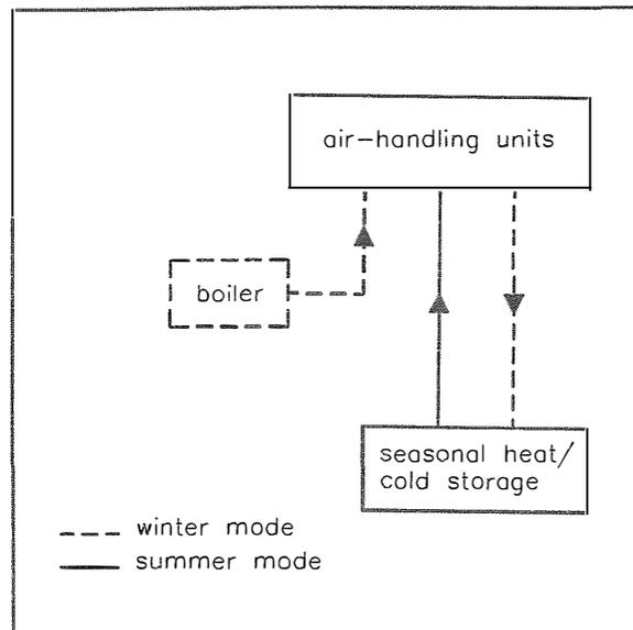
Fig. 3: Combined storage of cold and heat for the buildings sector
