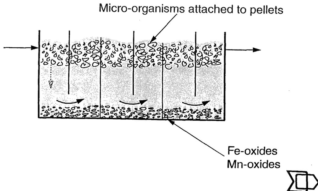
Figure 4 Schematic depiction of a bioreactor.
