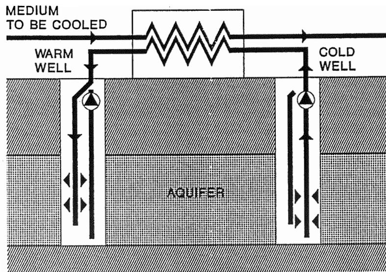
Figure 1 Working principle of an aquifer thermal energy storage system.
