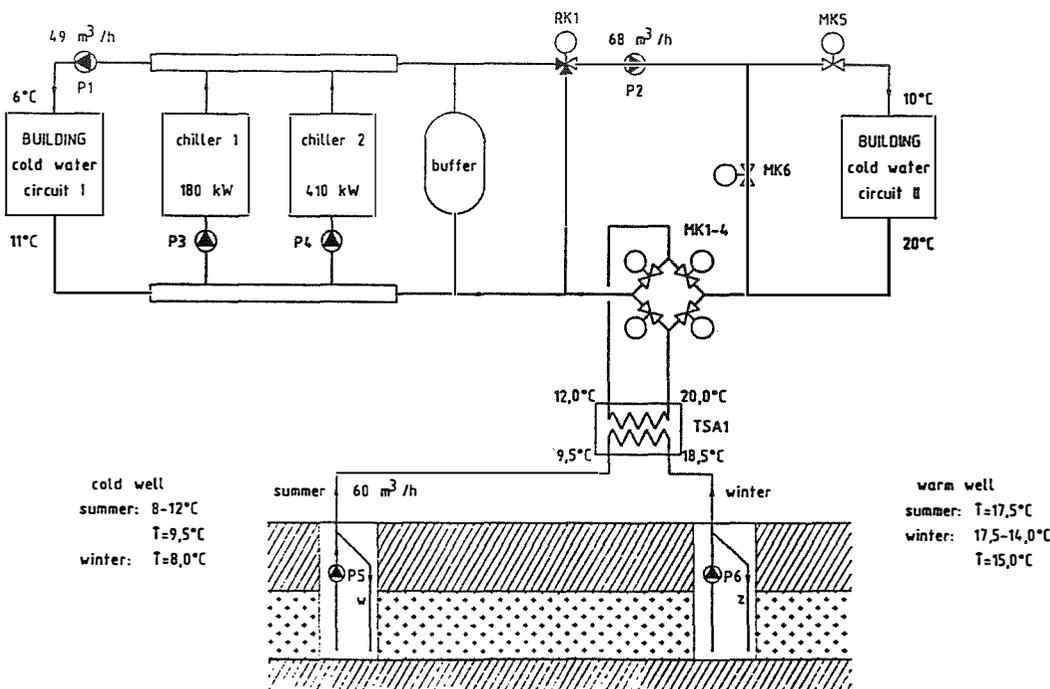
Figure 2 The ATES system integrated in the cooling system of the Bleuland Hospital.
